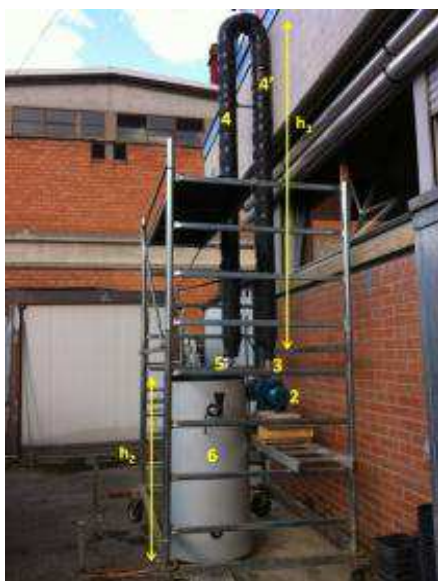
Fig.1 Experimental installation with 300 liters thermally isolated tank in Florence, Italy.
